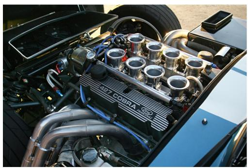
A fully built 427 CID Windsor Ford "small-block" fitted with an eightstack, Fast controlled, fuel injection system makes it one of the easiest driving, most flexible combinations for both road and track.
