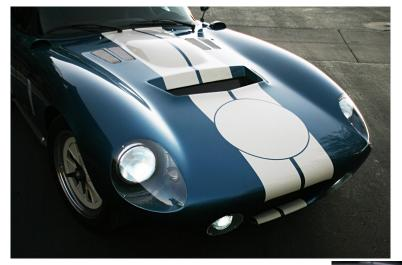
BRE headlight and driving light lens covers with custom stainless steel flush-fitted mounting hardware, just like the original racers
